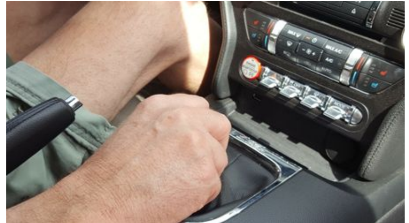
3rd to 4th Gear; Note: depending on your hand position during the 3rd to 4th motion this will result in pulling the shifter toward your hip. You might end up grabbing 2nd gear instead - OUCH!
