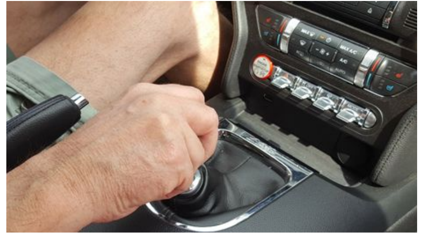
1st to 2nd Gear (note that using this grip your hand will pull the shifter towards your hip).
